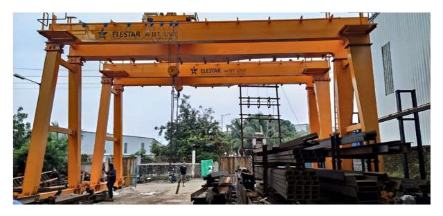
Gantry cranes are same as the regular overhead cranes except that the bridge for carrying the trolley is rigidly supported on two or more legs running on fixed rails or other runway. These "legs" eliminate supporting runway and columns and connect end trucks which run on a rail, either embedded in or laid on top of the floor.
